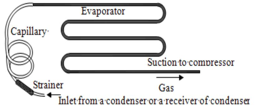
Physically the capillary tubes are hollow tubes made with drawn copper, with internal diameters ranging between 0.51 and 2 mm
